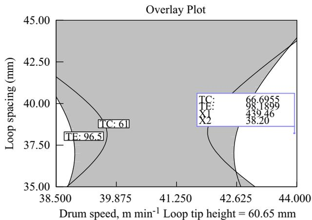
Fig. 12 – Superimposed contours for threshing capacity (TC, kg h<sup>-1</sup>) and threshing efficiency (TE, %) at varying drum speed (m min<sup>-1</sup>) and loop spacing (mm) at fixed loop tip height of 60.65 mm.
