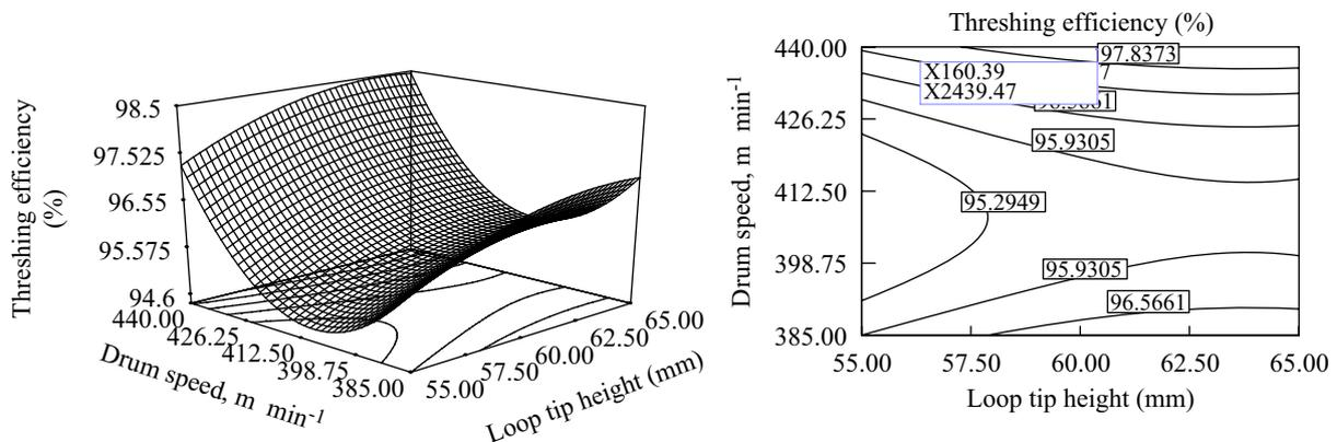
**Fig. 9 – Effect of drum speed ( $\text{m min}^{-1}$ ) and loop tip height (mm) on the threshing efficiency (%) at optimum loop spacing of 39.1 mm.**
