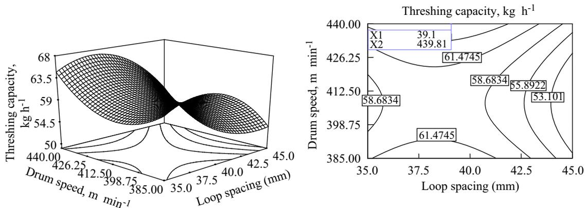
Fig. 5 – Effect of drum speed (m min<sup>-1</sup>) and loop spacing (mm) on the threshing capacity (kg h<sup>-1</sup>) at optimum loop tip height of 61.6 mm.
