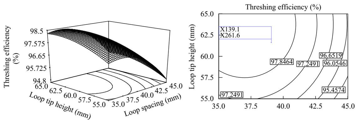
Fig. 7 – Effect of loop spacing (mm) and loop tip height (mm) on the threshing efficiency (%) at optimum drum speed of 439.46  $m\ min^{-1}$ .
