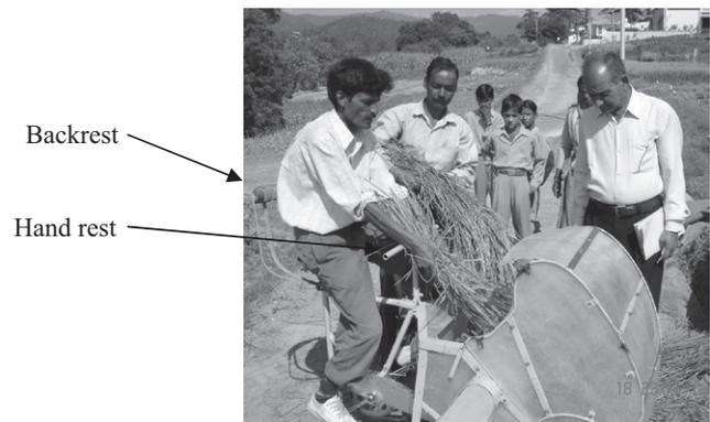
**Fig. 3 - VL paddy thresher in operation.**
