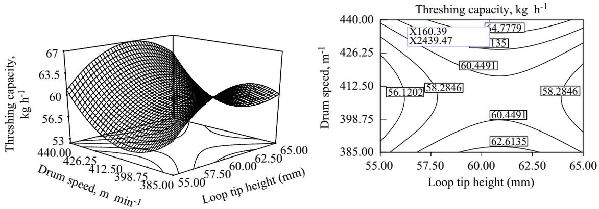
Fig. 6 – Effect of drum speed ( $m\ min^{-1}$ ) and loop tip height (mm) on the threshing capacity ( $kg\ h^{-1}$ ) at optimum loop spacing of 39.1 mm.
