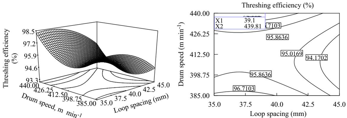
**Fig. 8 – Effect of drum speed ( $\text{m min}^{-1}$ ) and loop spacing (mm) on the threshing efficiency (%) at optimum loop tip height of 61.6 mm.**
