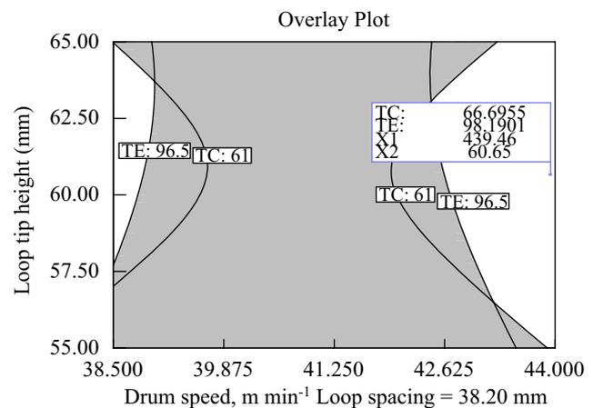
**Fig. 11 – Superimposed contours for threshing capacity (TC, kg h<sup>-1</sup>) and threshing efficiency (TE, %) at varying drum speed (m min<sup>-1</sup>) and loop tip height (mm) at fixed loop spacing of 38.20 mm.**
