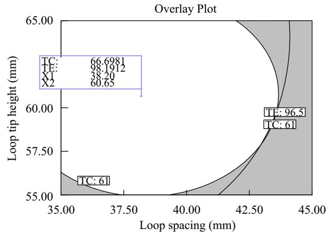
**Fig. 10 – Superimposed contours for threshing capacity (TC,  $\text{kg h}^{-1}$ ) and threshing efficiency (TE, %) at varying loop spacing (mm) and loop tip height (mm) at fixed drum speed of  $439.46 \text{ m min}^{-1}$ .**
