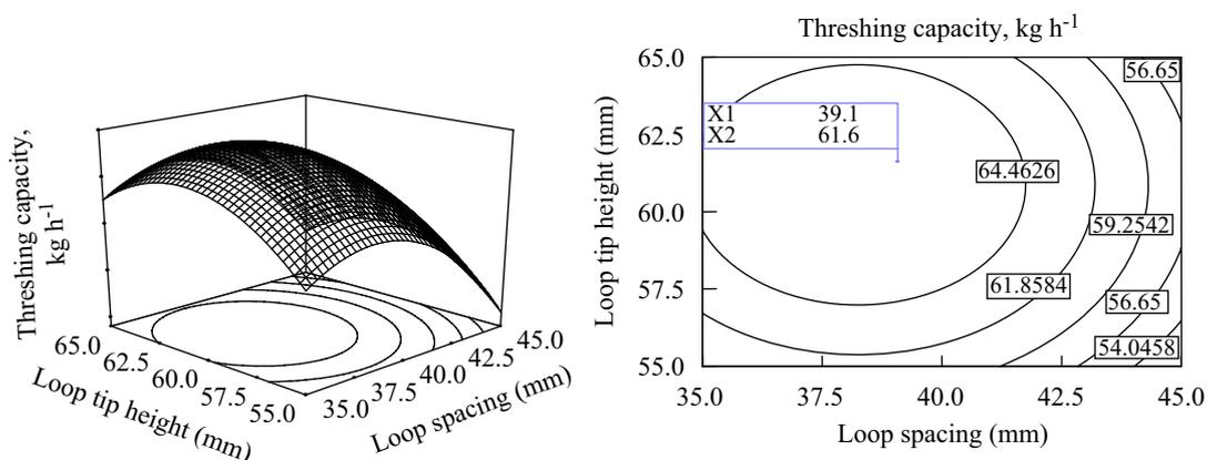
Fig. 4 – Effect of loop spacing (mm) and loop tip height (mm) on the threshing capacity ( $\text{kg h}^{-1}$ ) at optimum drum speed of  $439.46 \text{ m min}^{-1}$ .
